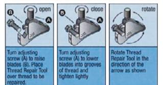
Turn adjusting screw (A) to raise blades (B) face Thread Repair Tool over thread to be repaired.
